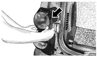
3. Unlock and remove electrical connector.
